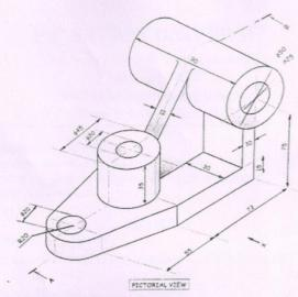
Q-3 Draw the Isometric Drawing of the following object.
